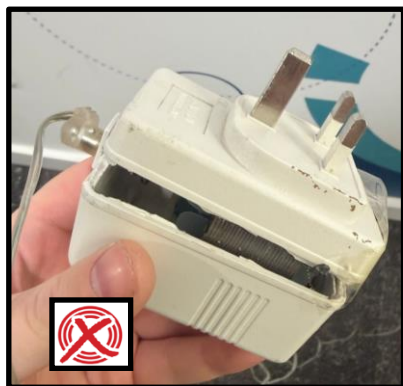
Damage to plug casing (Visual check)
